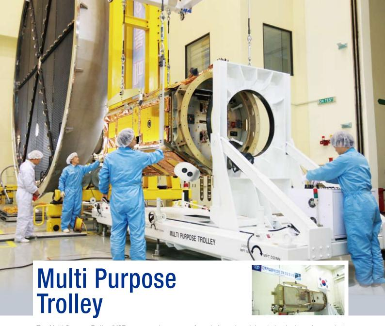
The Multi Purpose Trolley (MPT) supports the spacecraft or dedicated modules during horizontal or vertical integration and provides a table capable of tilting and rotating the spacecraft to any attitude between spin axis vertical and horizontal.
